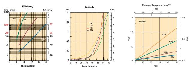
Results typical from Multi-pass tests run per test standard ISO 16889 @ 30 gpm to 100 psid terminal - 10 mg/L BUGL Refer to Appendix on pages 227-228 for relationship to test standard ISO 4572.
