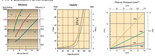
Results typical from Multi-pass tests run per test standard ISO 16889 @ 45 gpm to 100 psid terminal - 10 mg/L BUGL Refer to Appendix on pages 227-228 for relationship to test standard ISO 4572.
