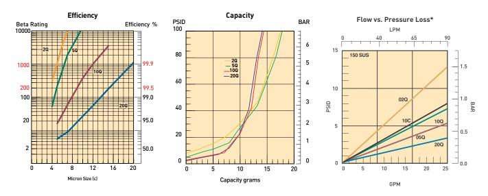
Results typical from Multi-pass tests run per test standard ISO 16889 @ 15 gpm to 100 psid terminal - 10 mg/L BUGL Refer to Appendix on pages 227-228 for relationship to test standard ISO 4572.
