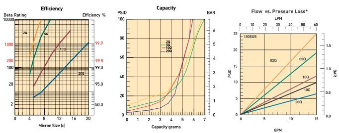
Results typical from Multi-pass tests run per test standard ISO 16889 @ 10 gpm to 100 psid terminal - 10 mg/L BUGL Refer to Appendix on pages 227-228 for relationship to test standard ISO 4572.
