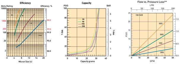
Results typical from Multi-pass tests run per test standard ISO 16889 @ 15 gpm to 100 psid terminal - 10 mg/L BUGL Refer to Appendix on pages 227-228 for relationship to test standard ISO 4572.
