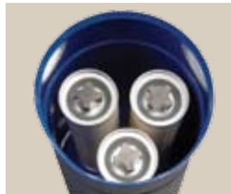
The elements are installed in the housing. They are held in place by a center rod and threaded end cap. This design allows for easy element changeout. The inlet is on the bottom of the housing and the air flows from the inside to the outside. The coalesced liquid collects at the bottom of the internal separator plate and can be easily drained away.
